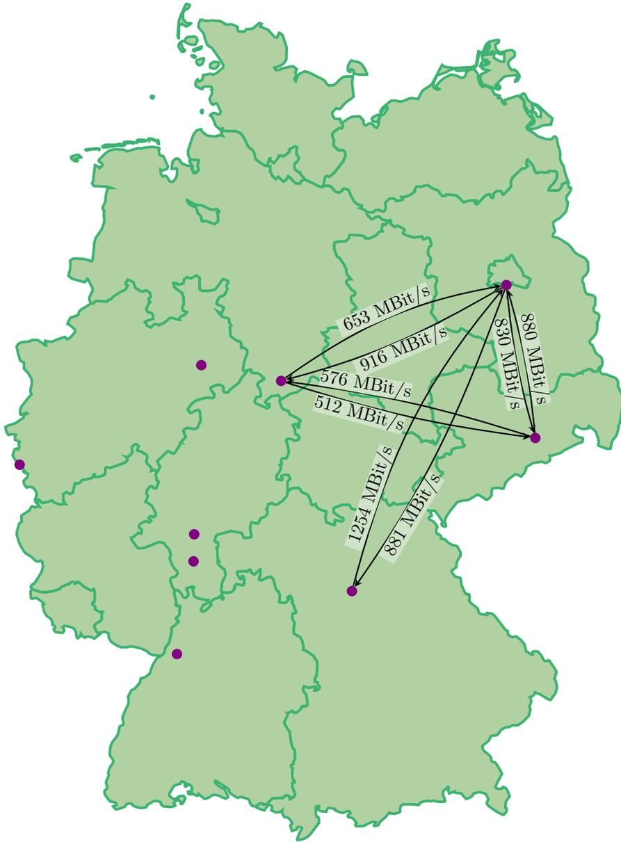
Figure 2: NHR centers in Germany and the maximum bandwidth between them as measured in the data transfer experiments.
